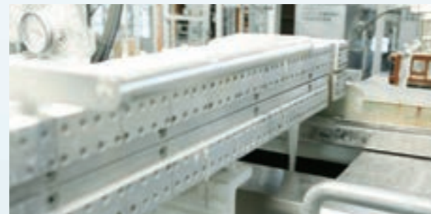
Pellet production process in the powder paint factory. The mixed powder is cooled down to about 30°C by the cooling equipment.
