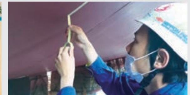
Nippon Paint Marine Coatings engineer checking the state of a FASTAR coating
