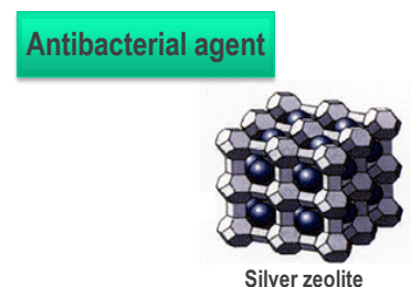
Active ingredients fixed in the pore
